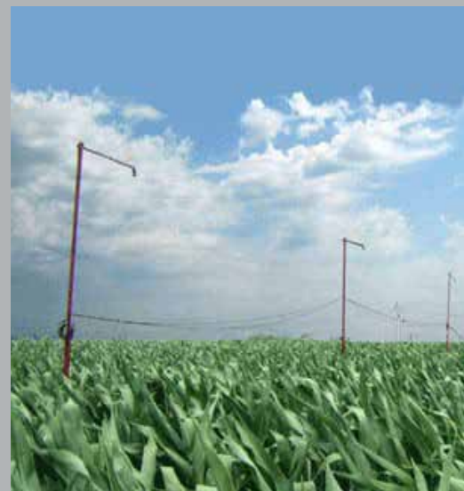
Field setup used to install two infrared thermometers above the crop canopy. One sensor was pointing east and another was pointing west.
