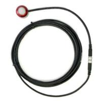
Inline cable connectors are installed 30 cm from the sensor head (pyranometer pictured).
