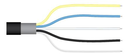
Yellow: Positive (signal from red sensor) Blue: Negative (signal from red sensor) White: Positive (signal from far-red sensor) Black: Negative (signal from far-red sensor) Clear: Shield
