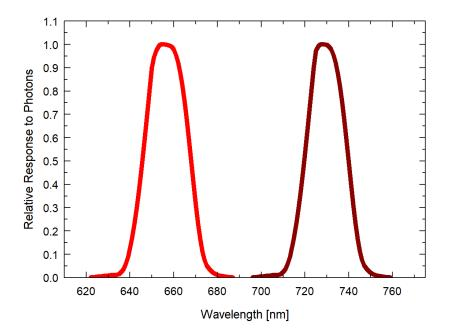
Mean spectral response measurements of six replicate red - far-red sensors (red sensor is centered near 655 nm, far-red sensor is centered near 730 nm). Spectral response measurements were made at 2 nm increments across a wavelength range of 600 to 800 nm in a monochromator with an attached electric light source. Measured spectral data from each sensor were normalized by the measured spectral response of the monochromator/electric light combination, which was measured with a spectroradiometer.
